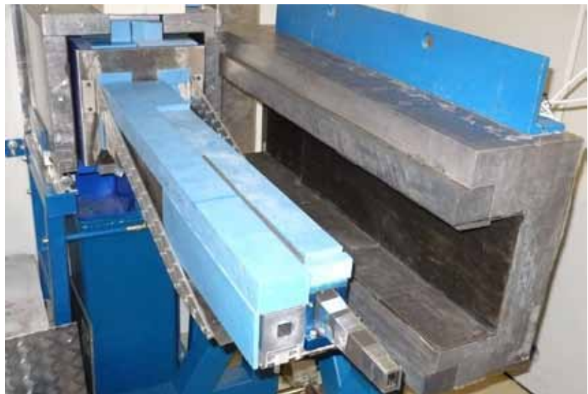
Fig. 2: Beam collimator and elliptical neutron guide, shielded.
