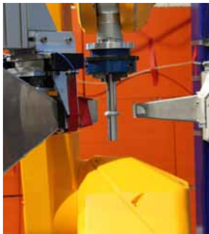
Fig. 1: Rotary friction welded sample of Al7020 and steel 316L.
