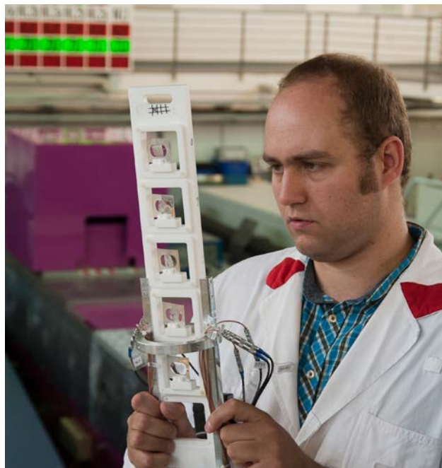
Josef Lichtinger examines the lithium distribution in brain samples. In his hands, he holds the self-developed detector with the tissue sections.
