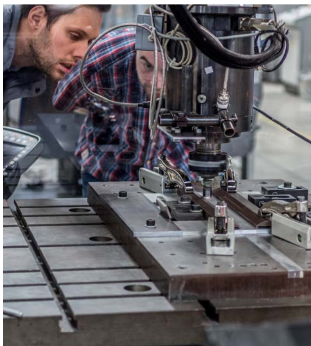
Dr. Andreas Bachmann (left) watches through safety glass as the robot welds two metal plates together with the rapidly rotating welding pin.
