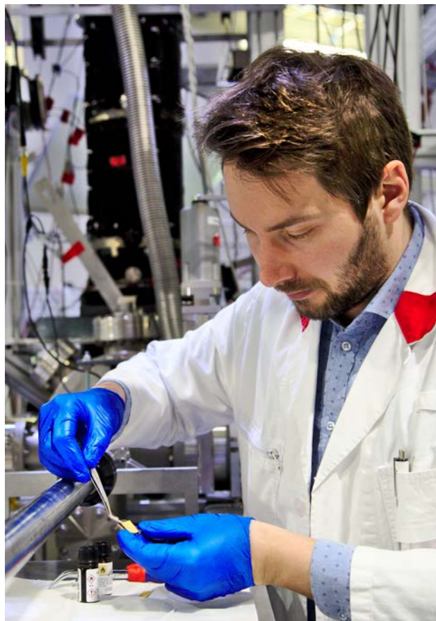
Dr. Marcel Dickmann places the membrane on a sample plate to study it using positron annihilation lifetime spectroscopy.
