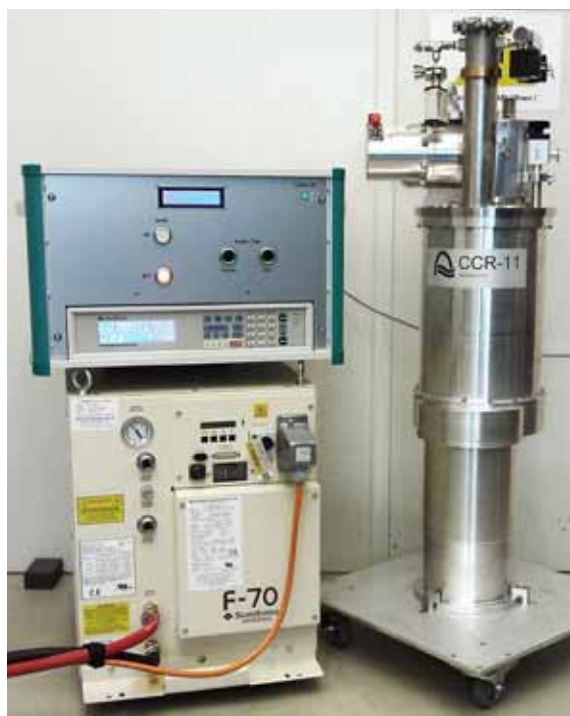
Figure 6: Closed cycle refrigerator (CCR) (right) with the newly developed universal control box (top left).
