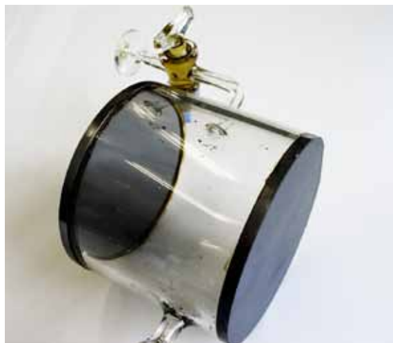
Figure 2: ^3\text{He} filter cell with beam windows made from single crystal silicon.
