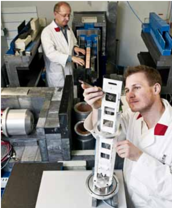
Figure 1: A moving mechanism changes the beam collimator and the elliptical neutron guide (back part) at the PGAA.
