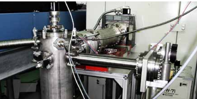
Figure 1: Experimental setup (partially dismantled) at MEPHISTO. The sample cell is placed inside the stainless steel vacuum chamber on the left side and irradiated by cold neutrons arriving from the back side of the picture. UCN are extracted perpendicularly to the incoming beam, and guided to a detector (not shown).
