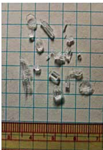
Figure 1. Photograph of mixed crystals. A single crystal of good shape (located center) was selected using a polarized microscope and used for neutron diffraction experiments.
