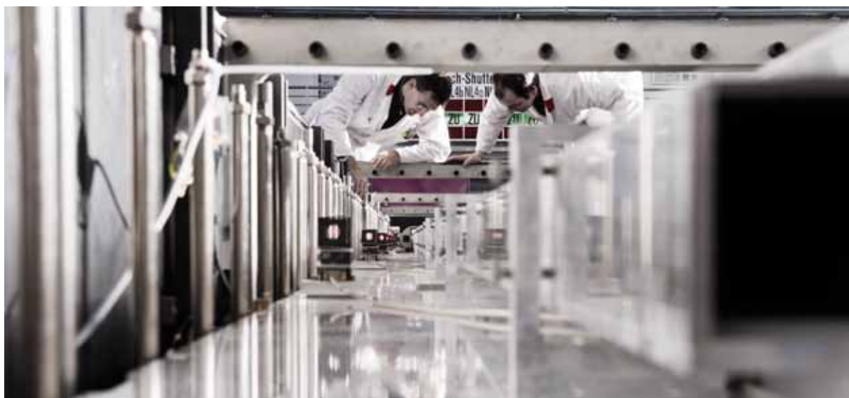
Figure 6: The SANS-1 team working on the collimation of the small angle scattering instrument. The laser system is visible on the left.
