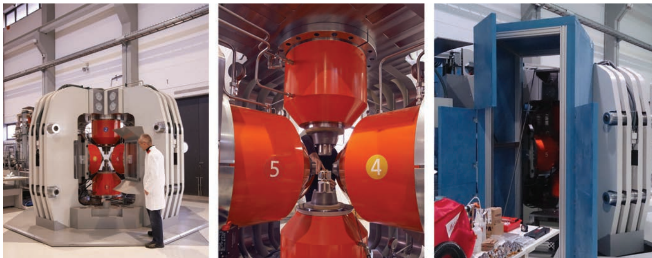
Figure 21: (left) View of the three-axis press before attachment of the detector frames. (middle) The stack of secondary anvils with the sample assembly is placed between the primary anvils before compression. (right) Installation of the detector frame and the instrument shielding for the left 90° detector bank.
