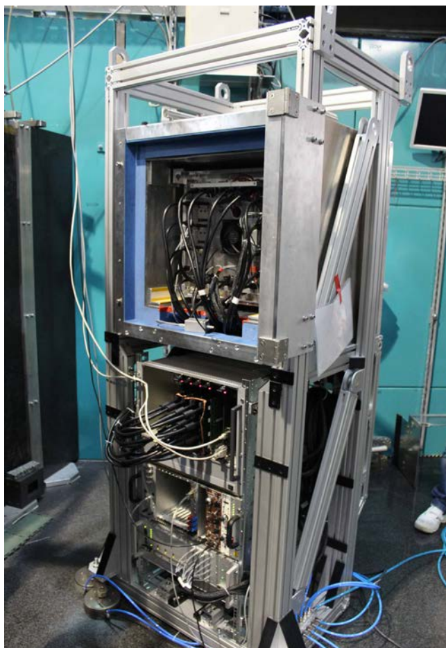
Figure 17: The back face of the new STRESS-SPEC detector in its housing before being closed for the commissioning tests.
