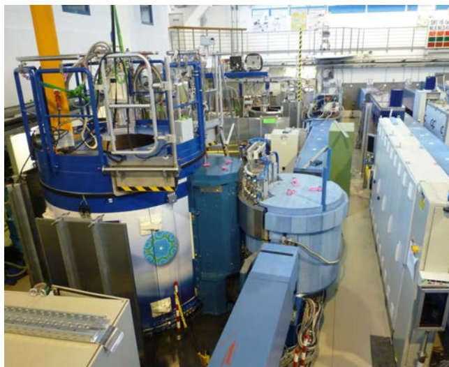
Figure 27: The new monochromator drum and the neutron velocity selector at DNS.
