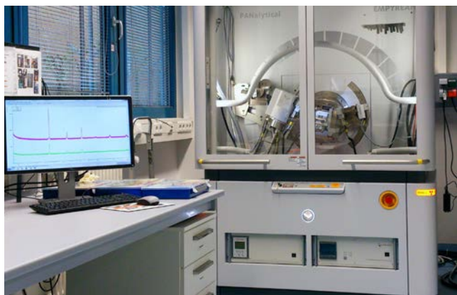
Figure 15: The new Empyren X-ray Diffractometer has been part of the Materials Science Lab equipment since August 2014.
