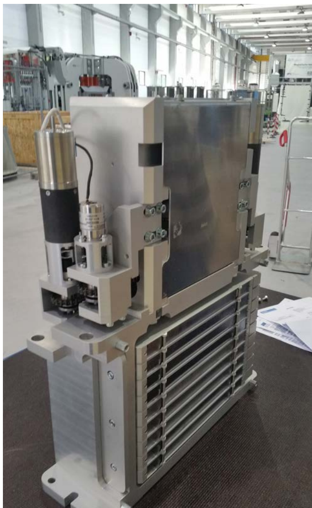
Figure 4: The Si 311 monochromator for POLI.
