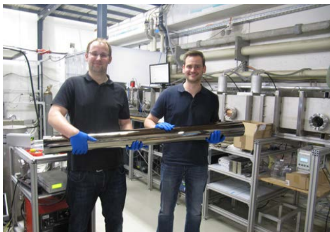
Figure 24: Hands on the first 1.5m long UCN guide element produced at the MLZ.
