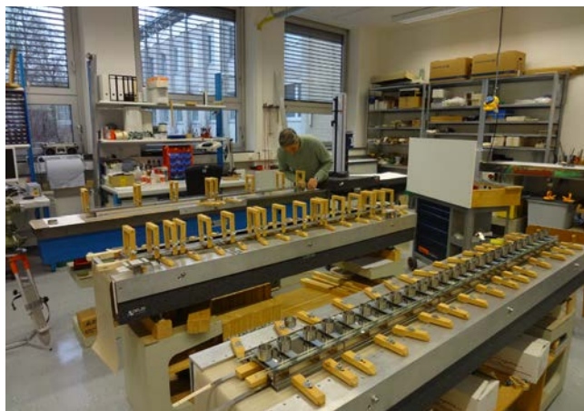
Figure 1: The new neutron guide assembly workshop: Josef Weber working on a two channel neutron guide element.
