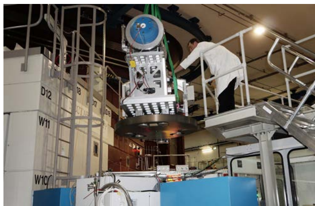
Figure 6: Crane transport of the POLI diffractometer to its new "home" on the beam line SR9a.
