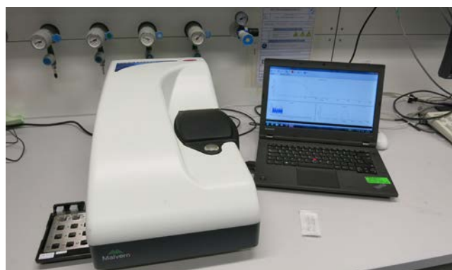
Figure 16: Picture of the Malvern Zetasizer Nano dynamic light scattering instrument. It can be operated from a lap-top computer.
