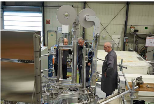
Figure 1: Mock-up on a 1:1 scale of the future Mo-99 irradiation facility made of stainless steel.
